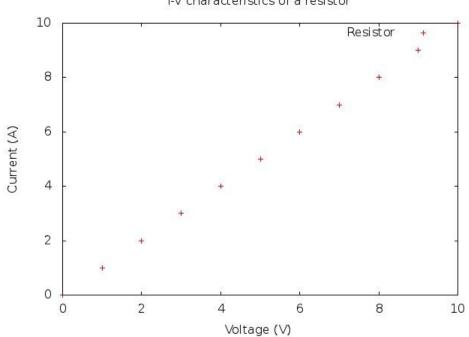
I-V characteristics of a resistor
